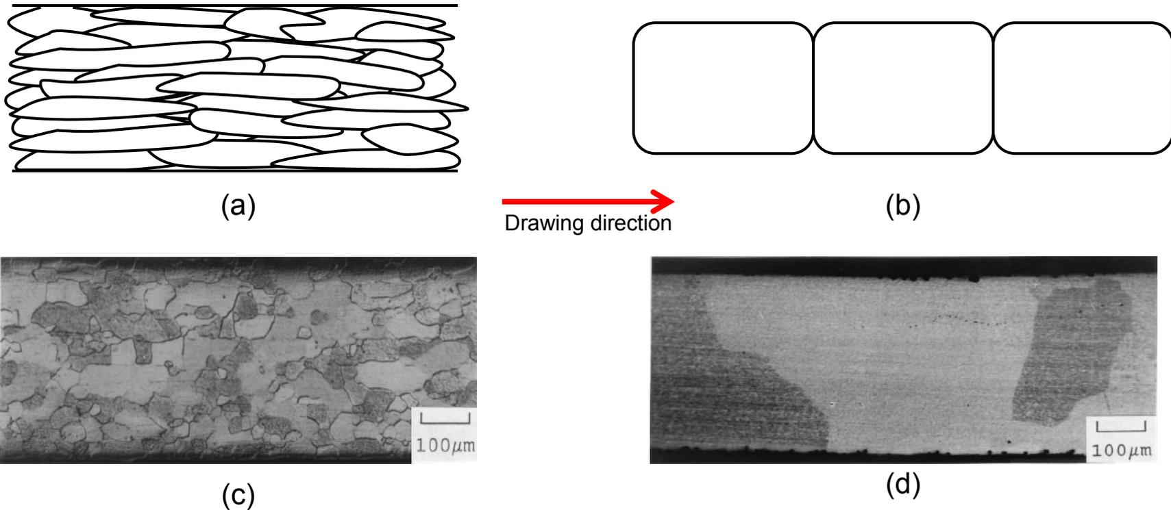
Schematic microstructures of (a) drawn W wire and (b) such a wire following high-temperature exposure. Figures (c) and (d) are light optical micrographs of W before and after high-temperature exposure.
