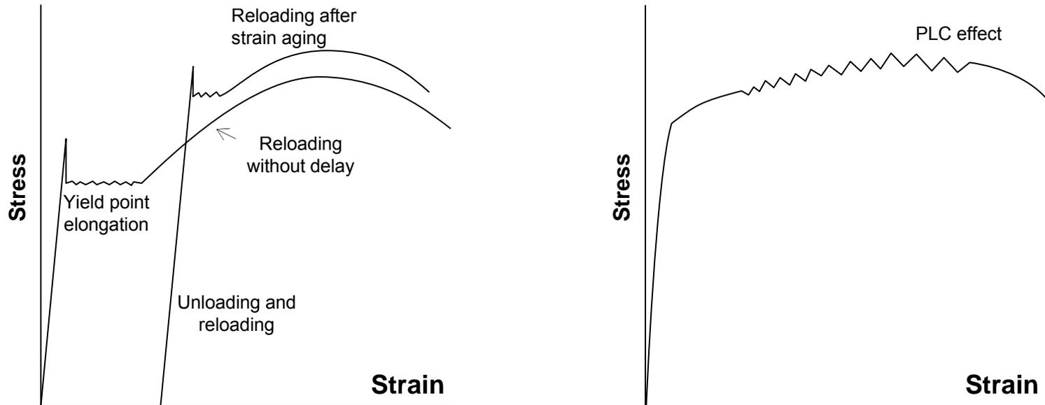
Schematic illustrations of (a) upper yield point formation characteristic of static strain aging and (b) serrated yielding characteristic of dynamic strain aging.
